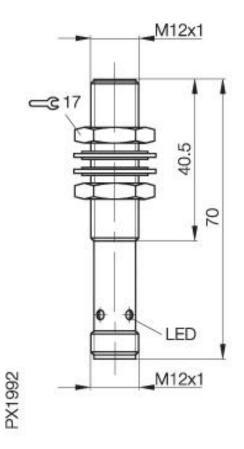
**Inductive Sensors** BES 515-325-S 4-C M12x1 x 70 normally-open Sn=2mm shielded
